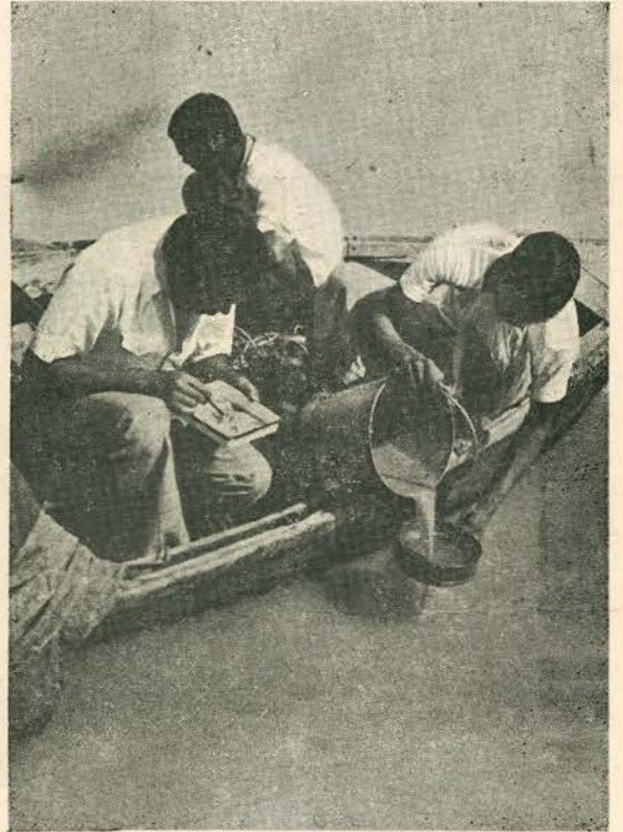
Fig. 12 Sieving the bottom samples through No. 40 brass sieve
