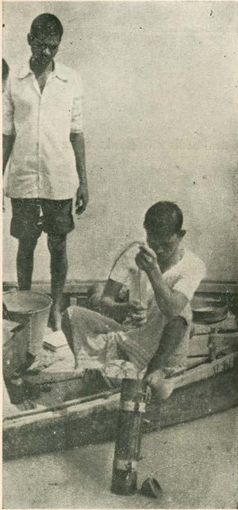
< Fig. 7 Collecting water samples with Von Dorn's Sampler
